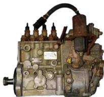
**Cummins 3.9L 4BT Inline Fuel Pump**
