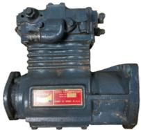
**Mack Bendix TuFlo 550 / 750 Air Compressor Core**
