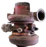
**Cummins / Holset HE551V Turbocharger Core**
